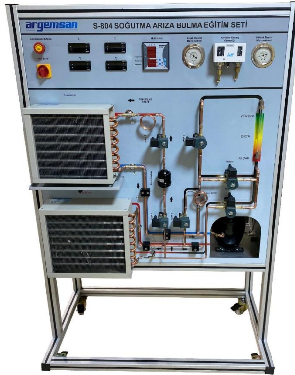
Vapor Compression Refrigeration Cycle Performance Analysis Experimental Setup
